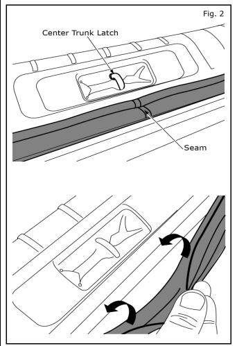
b) Locate seam on seal to center trunk latch.
