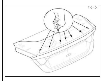
Locate punch marks in center of printed hole locations. A light, quick impact on center punch is recommended to prevent a deep dent on trunk lid. Seven (7) places total.
